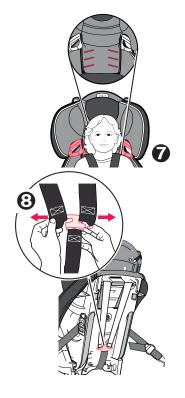
7. Pull strap ends through slots at front of seat ② and reinsert them in the desired slots ③. Check that the straps are not twisted.
